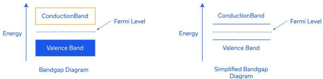
Figure 5: Simplified band gap diagram showing the top of the valence band and bottom of the conduction band.
