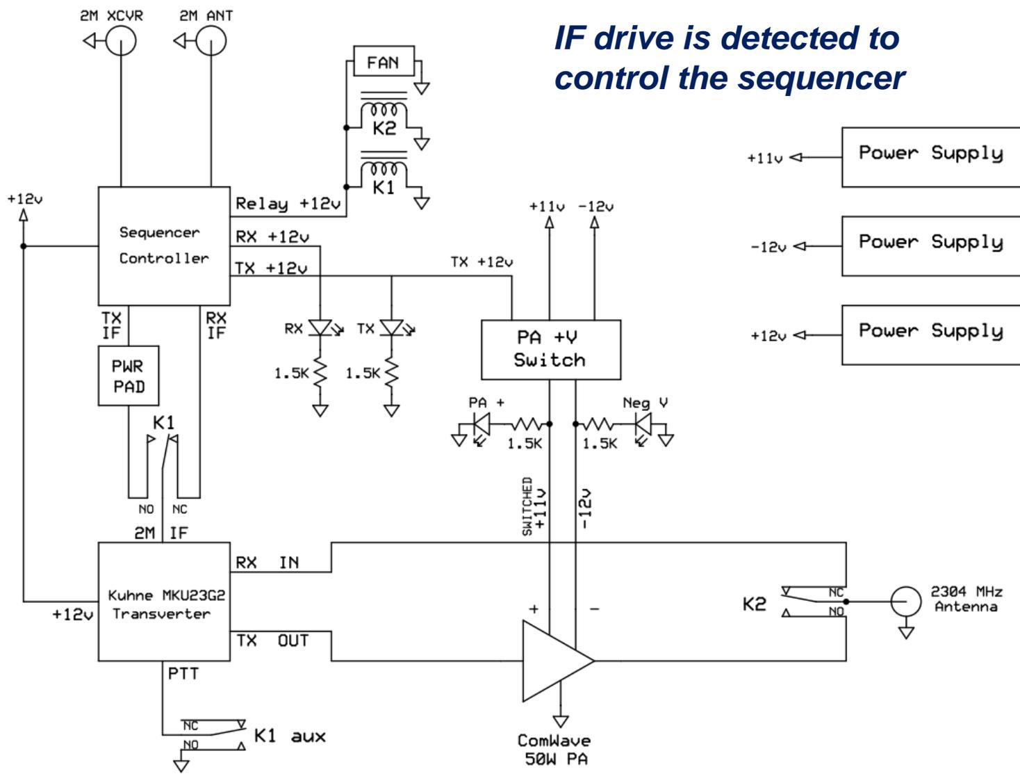
*IF drive is detected to control the sequencer*
