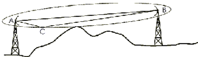
Figure 6 Fresnel Zone for a Radio Link
