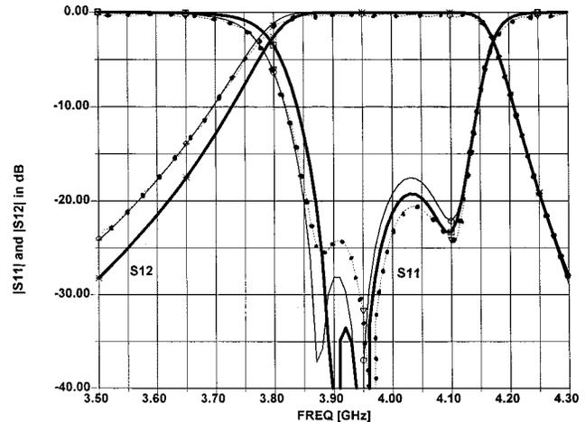
Fig. 2. Dots show the measured responses of the filter in Fig. 1 while the narrow solid lines show the 3D planar CAD results with the actual  $A_o = 25.6$ ,  $B_o = 51.2$  mm housing dimensions. The heavy solid lines show 3D planar CAD results if  $A_o = 12.8$ ,  $B_o = 25.6$  mm are assumed instead.
