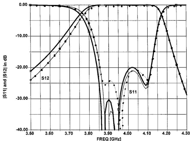
Fig. 5. Dots above show the measured response for the filter while the heavy solid lines show the response obtained utilizing 2D + 1 CAD with  $A_o = 25.6$  mm in Fig. 4 with  $f_{\text{calc}} = 3.95$  GHz (i.e., line parameters are calculated at the center of the passband). The narrow solid lines show the 2D + 1 CAD results if we replace  $A_o = 25.6$  with  $A'_o = 13.8$  mm in Fig. 4.
