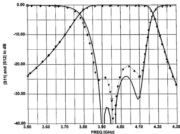
Fig. 6. Dots above show the measured response while the solid lines show the response computed using 2D + 1 CAD with  $A_o = 25.6$  mm as in the actual filter, but with the line parameter computed using  $f_{\text{calc}} = 2.8$  GHz instead of 3.95 GHz.
