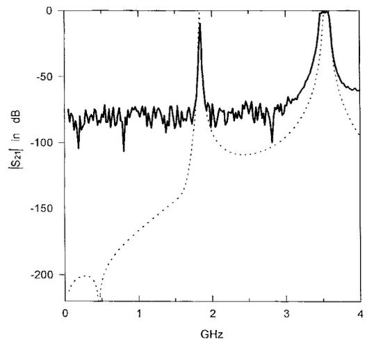
Fig. 10. Broad-range computed and measured responses for the trial four-resonator microstrip filter. The measured response is limited by the network analyzer dynamic range.
