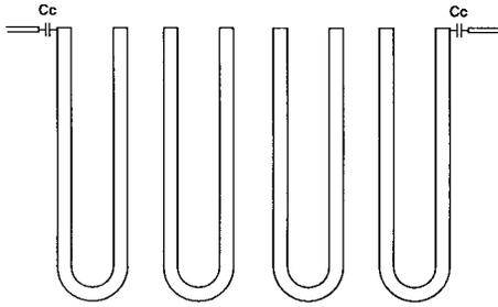
Fig. 8. A four-resonator hairpin-comb filter with capacitance couplings at its ends.
