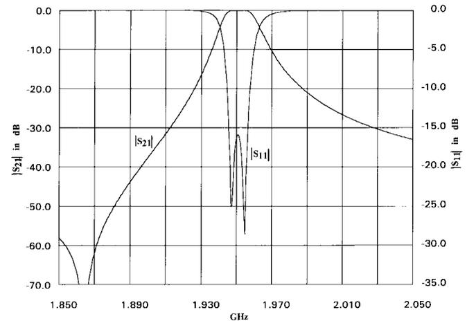
Fig. 7. A broad-range computed response for the two-resonator trial filter.
