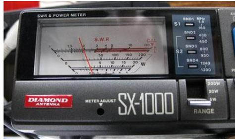
A Diamond SX-1000 meter can handle the 902 and 1296 MHz bands, but not really the microwave bands higher than that.
