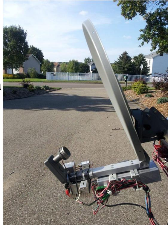
This bent dish had about 15 db less gain than it should have!
