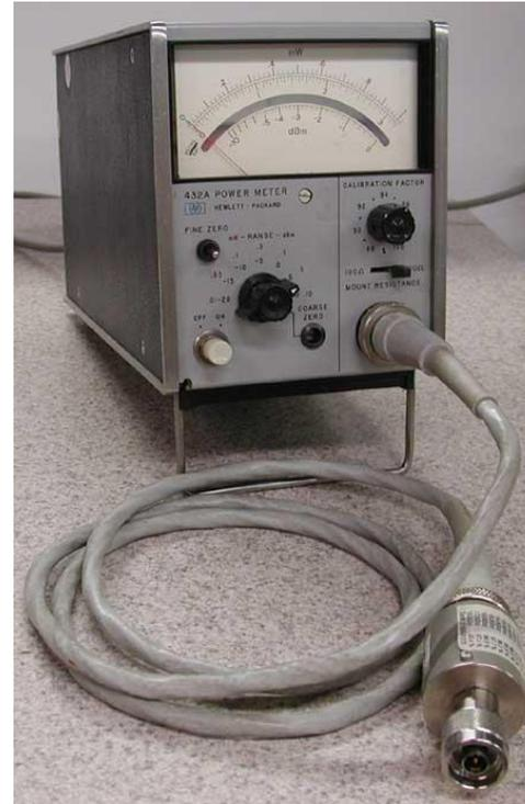
An HP432A power meter with an 8478B thermistor can measure 18 GHz RF frequencies easily and detect very low power levels (0.01 mW to 10 mW full scale – have you got an attenuator handy?)
