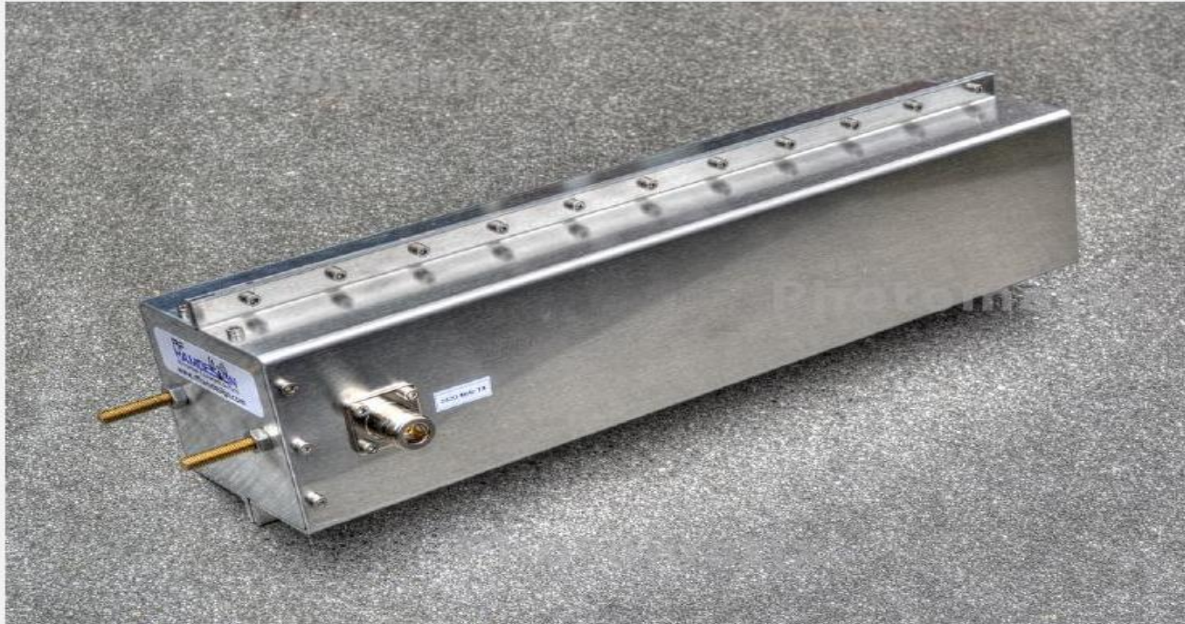
Dual Mode Circular Dish Feed 2320MHz
