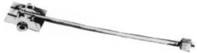
Figure 19. Photograph of 1/2" CQ Impedance Measurement Probe
