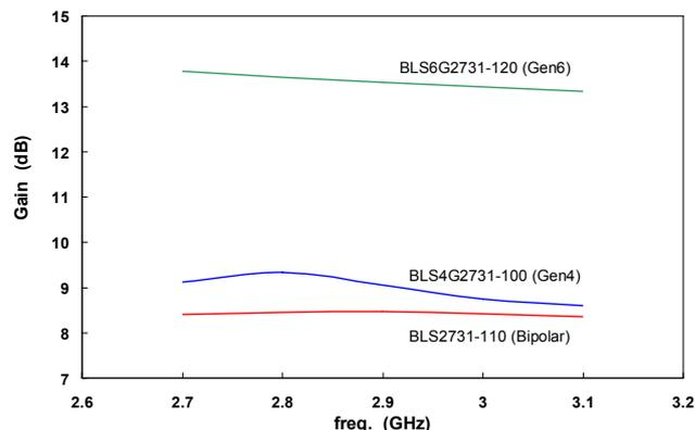
Figure 8: Gain comparison of broadband matched devices operating in the 2.7-3.1 GHz frequency band.
