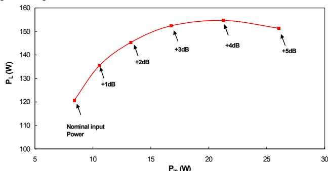
Figure 11: BLS6G3135-120 overdrive capability measured at 3.5 GHz,  $V_{ds} = 32$  V,  $I_{dq} = 100$  mA,  $t_P = 300\mu$ s,  $\delta = 10\%$ .
