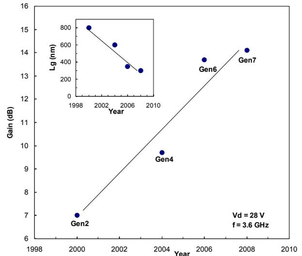
Figure 4: Gain improvement at  $f=3.6$  GHz for the subsequent LDMOS generations as measured by load pull techniques. The inset shows the reduction of the gate length.
