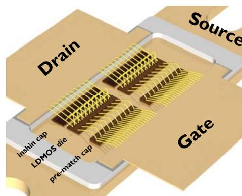
Figure 1: Picture of LDMOS devices in a ceramic package with internal pre and post matching.
