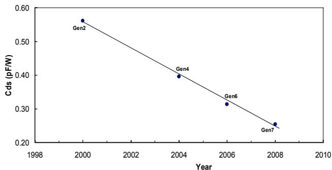
Figure 6: Reduction of off-state output capacitance at  $V_d = 28V$  for subsequent LDMOS generations.
