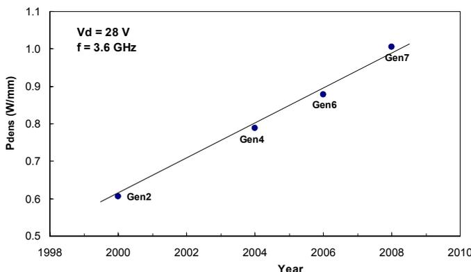
Figure 3: Evolution of the LDMOS power density at 3.6 GHz measured for packaged devices without internal matching in a load pull set-up.
