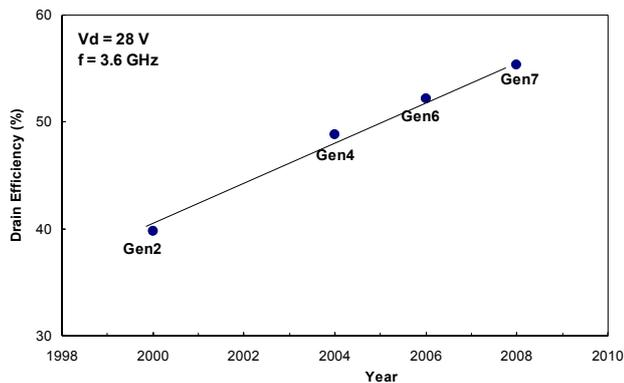
Figure 5: Evolution of LDMOS peak drain efficiency at 3.6 GHz for a supply voltage of 28 V.
