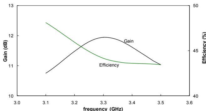
Figure 10: Gain and efficiency of the BLS6G3135-120.
