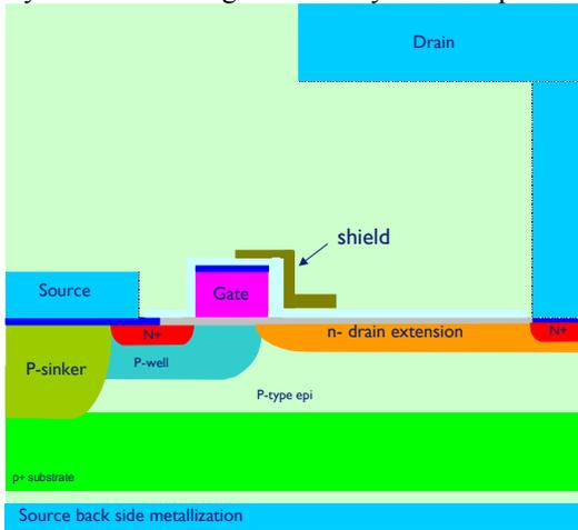
Figure 2: Schematic cross-section of state of art RF LDMOS fabricated in an 8 inch CMOS fab.
