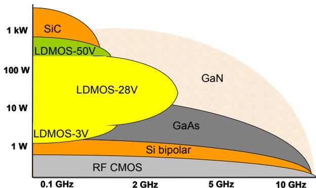
Figure 13: An overview of preferred transistor technologies for design-ins in the year 2008 as a function of power and frequency. LDMOS is continuously expanding towards higher power and frequency.
