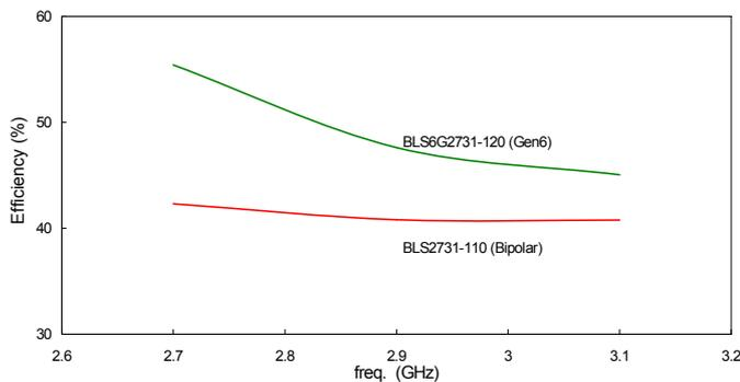
Figure 9: Drain efficiency comparison of broadband matched devices operating in the 2.7-3.1 GHz frequency band.
