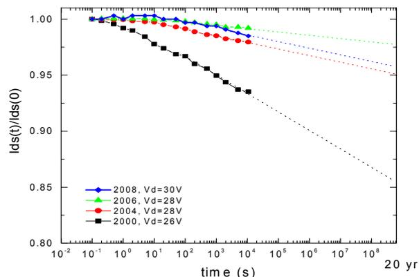
Figure 7: Degradation of the bias current as a function of time at room temperature. The LDMOS is biased at 26-30 V and a quiescent current of 5 mA/mm.
