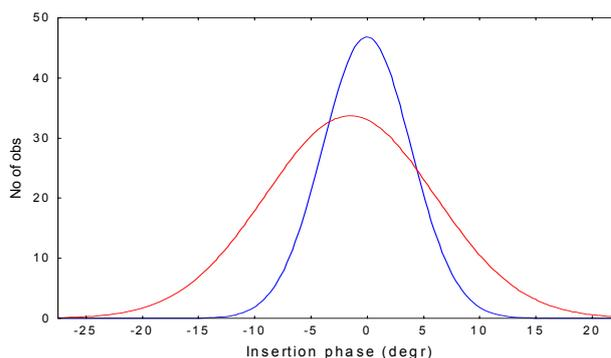
Figure 12: Batch to batch insertion phase distribution of both LDMOS and bipolar devices at S-Band frequencies.
