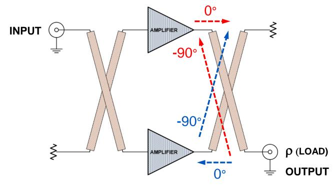
Power amplifier output match is for power not reflection; so, a single amplifier operating into a mismatch experiences multiple reflections due to mismatched source and load. This problem is mitigated in quad-combined amplifiers. Any reflected signal from the amplifier output is combined at the isolate termination.
