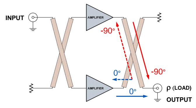
● Load mismatch is applied differently. Upper amplifier sees the load reflection shifted by -180° more than the lower amplifier. This desensitizes the pair. If one amplifier is more heavily loaded, the other is more lightly loaded. The total supply current is more constant. Note: Both amplifiers do see a mismatched load.
