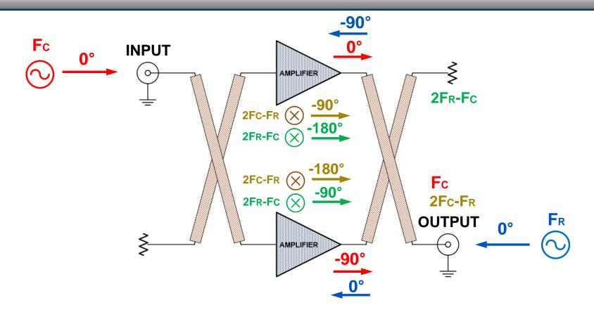
S Reverse IMD: 2FR-Fc is sent to the output isolate termination. Reverse IMD: 2Fc-FR is sent to the output Port. Conclusion: some reverse IMD is suppressed.
