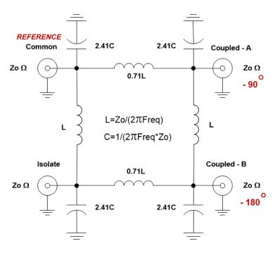
A lumped branchline hybrid uses an LC approximation of the branchline quarter-wave lines:
