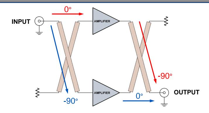
● The total phase shift through hybrids is -90° for each amplifier path to the output port. Both amplifier signals arrive in-phase at the output port.
