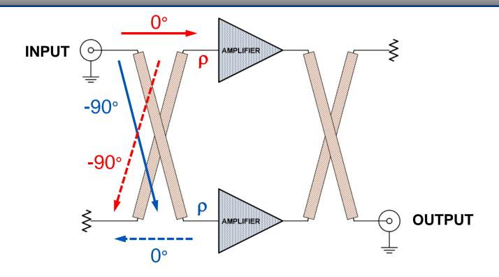
**2** Input from each amplifier is sent to the isolate termination. The path phase shift for each amplifier to the isolate termination is:  $\angle \rho$  - 90°. Input VSWR of the pair is 1:1.
