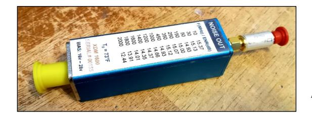
$$ENR = \frac{T_{hot} - T_{cold}}{T_o}$$
