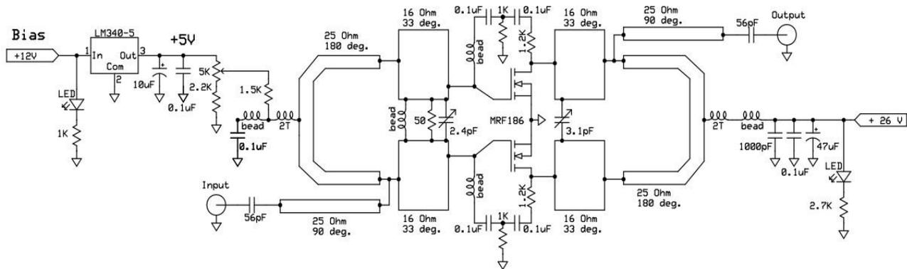
Figure 12 PA schematic
