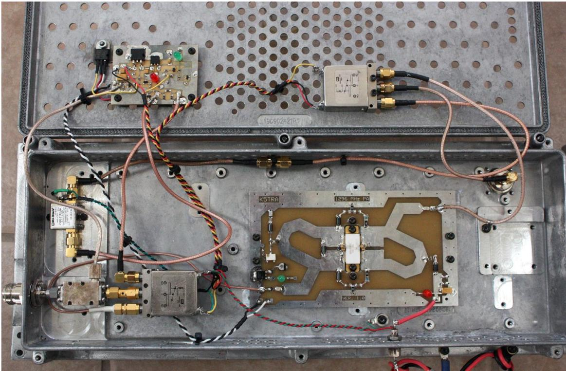
Figure 13 1296 MHz remote PA and LNA
