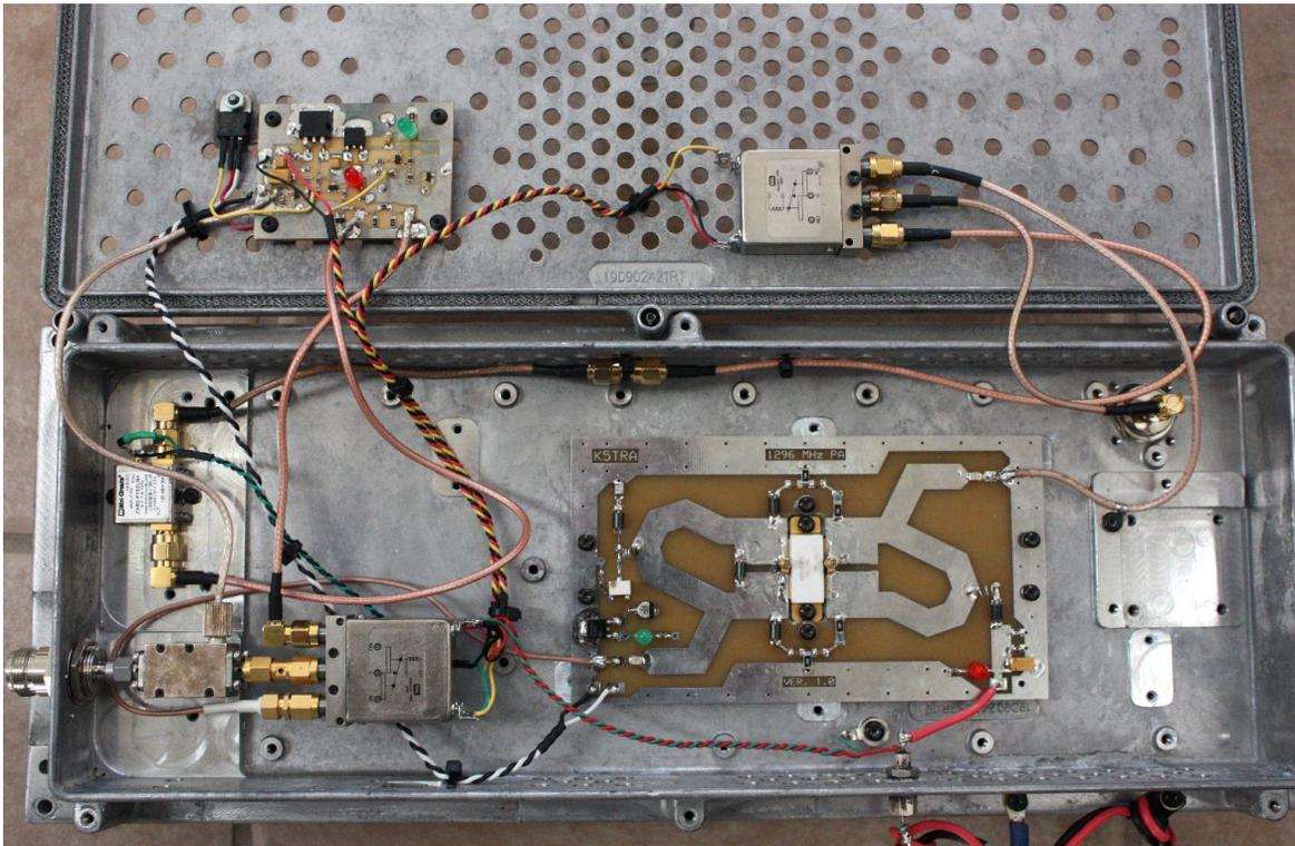
Figure 13 1296 MHz remote PA and LNA
